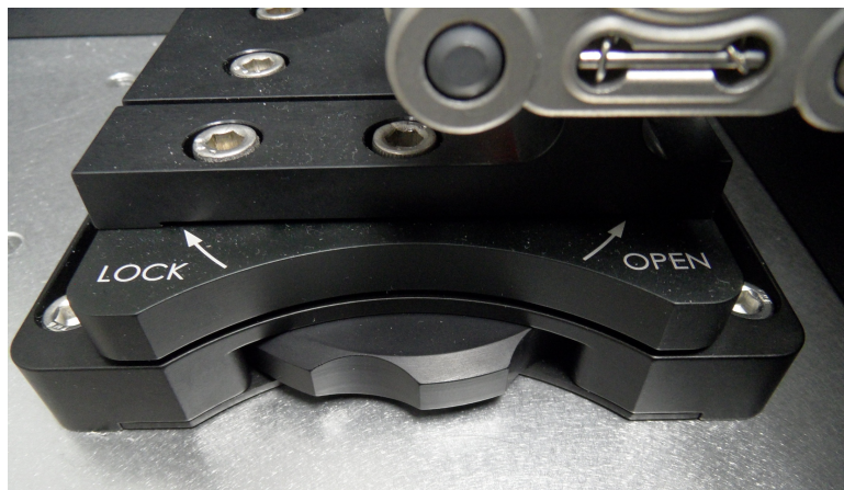
Figure 7 – Fixture locking and unlocking occurs through rotation of the locking wheel in the fixture baseplate. Rotate the wheel to the left to lock a fixture into place, and rotate the wheel to the right to unlock a fixture for removal from the baseplate.
