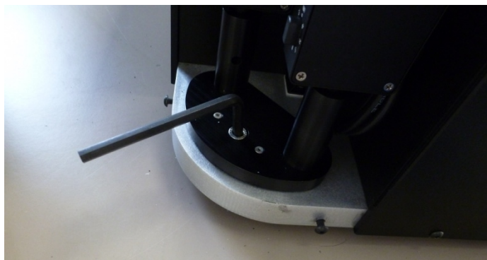
Figure 35 – Use a 5 mm Allen wrench to unmount the detector module from the baseplate. Fully remove the screw before removing the detector module.
