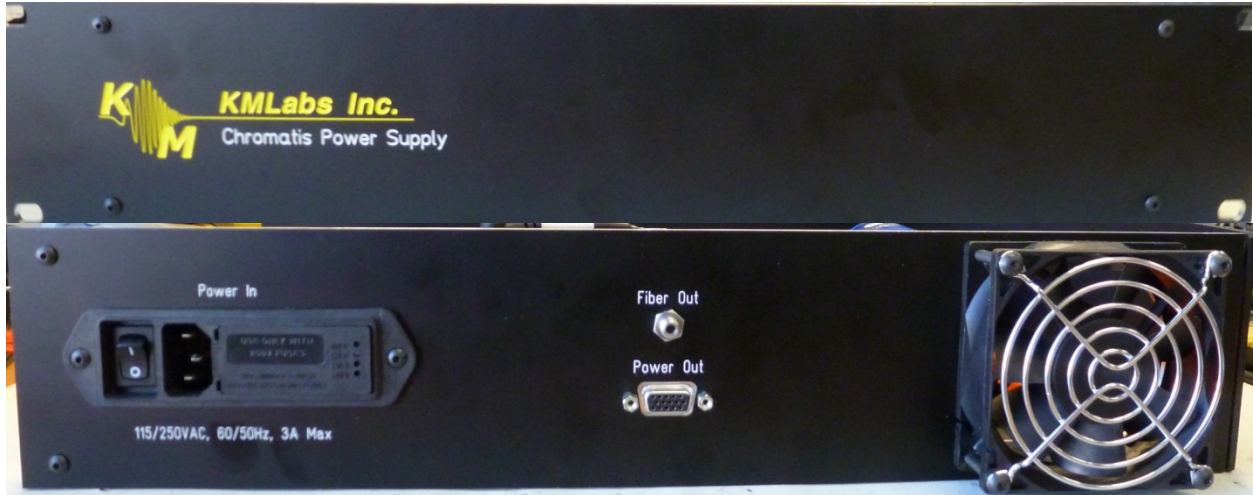
Figure 5 – Chromatis power supply front (upper picture) and back (lower picture). The power supply on-off switch is next to the power cord plug. The umbilical cables plug into the Fiber Out and Power Out ports.
