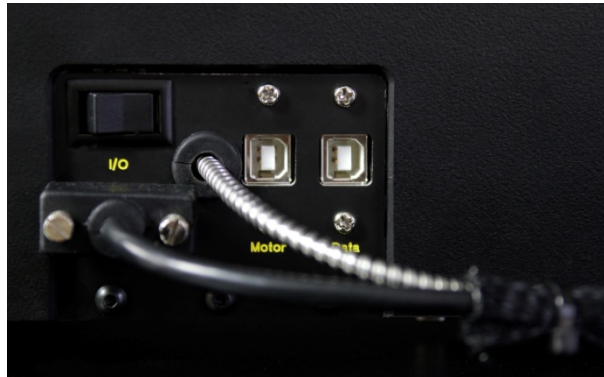
Figure 4 – Umbilical and data port. This panel also contains the instrument on-off switch. The on position is denoted by “I” and the off position is denoted by “O”. The silver cable is the fiber optic cable carrying the light from the various light sources to the instrument head. The black D-sub connector provides power and control for the various components of Chromatis. The USB Motor and Data connections are plugged directly into the included laptop computer.
