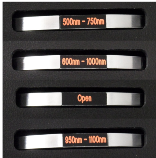
Figure 32 – Pictures of the four wavelength selection filter positions. Each position rotates one filter into the white light beam path. The filter labels indicate the approximate wavelength ranges that can be measured with each filter and the Silicon detector. Open indicates no filter.
