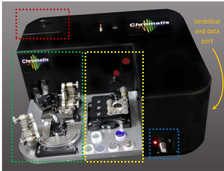
Figure 2 – Chromatis instrument head. The fixture being used for the current measurement is installed in the measurement area (outlined in yellow). The other fixtures are locked to the baseplate in the fixture storage area (outlined in green). The detectors are contained in a user-accessible section (outlined in red), and two detector options are available. The light selection switch also is shown on the front of the device (outlined in blue). The umbilical and data port is on the side indicated by the arrow.
