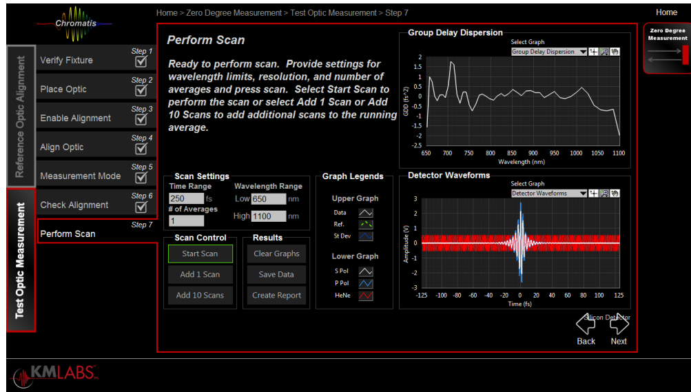
Figure 19 – Results of the initial scan showing interference patterns are detected properly (bottom right). The user now can choose the scan settings that are appropriate for the optic under test.
